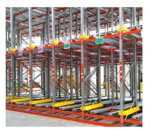
Variant : push-back pallet racks. Loads and unloads from the same side. When a pallet is added, it pushes back the pallets already stored on the same row.
